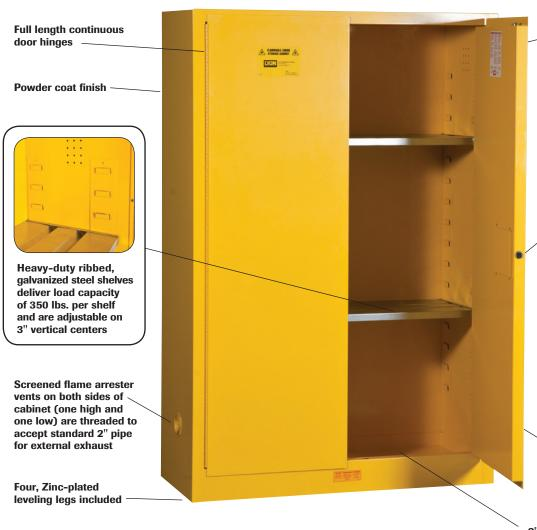
All-welded 18-gauge, double wall construction with 1½" of insulating air space offers fire resistant protection
