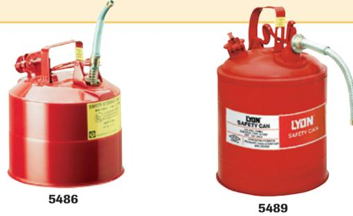
**Type II Safety Cans** have two openings (one pouring, one filling). Flexible metal nozzle effectively dispenses into small openings and eliminates need for funnel, providing ground path to prevent static sparks.
