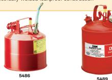
**Type II Safety Cans** have two openings (one pouring, one filling). Flexible metal nozzle effectively dispenses into small openings and eliminates need for funnel, providing ground path to prevent static sparks.
