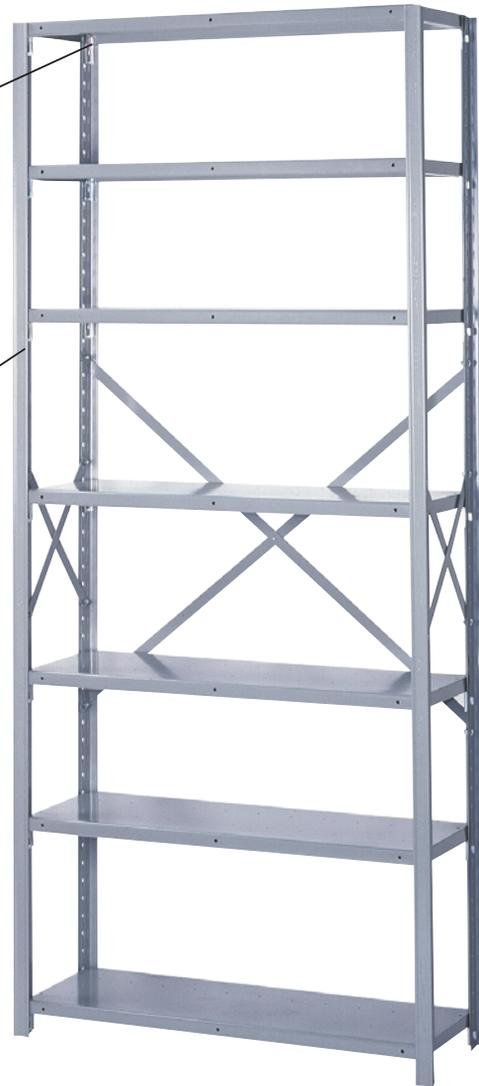
\*Capacities are based on evenly distributed loads. All shelves maintain a 1.65 safety factor and posts a 1.92 factor. See page 39 for detailed product specifications. Maximum load capacity per section is 8,000 lbs. based on 18" maximum shelf spacing and no seismic considerations.
