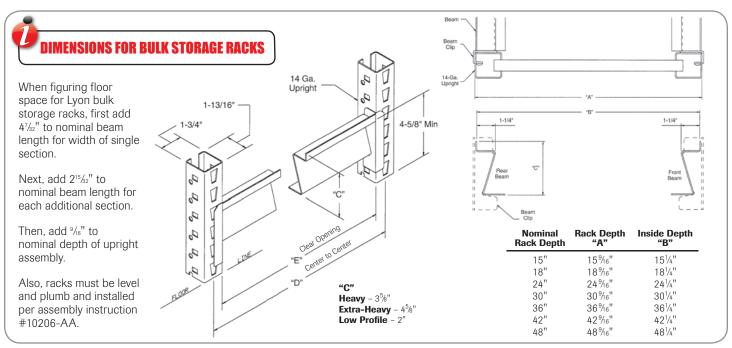
Capacities shown are maximum safe evenly distributed static loads per pair of beams with front-to-back support. Upright capacities are based on beam centers no greater than 36"
