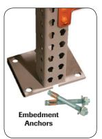
Bigfoot® Rack from Lyon gets its name from the oversized 8" x 6-1/2" x 3/8" all-welded footplate which anchors our 12-gauge steel, 55,000 psi upright posts. The 3" x 3" uprights are slotted to allow easy beam adjustment on 2" centers. 13-gauge bracing on 48" centers produces a structurally superior member with capacities up to 20,000 lbs.
